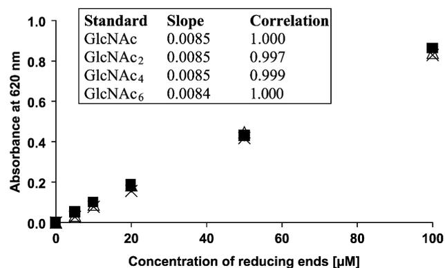
Fig. 2. Calibration of the MBTH method. The figure shows absorbance at 620 nm versus molar concentrations of GlcNAc (■), GlcNAc<sub>2</sub> (□), GlcNAc<sub>4</sub> (△) and GlcNAc<sub>6</sub> (×) in the 200 µl samples. The experiment was carried out in triplicate and the values represent the average. The insert shows the data for the regression lines.
